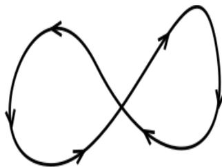
Fig. 5: To easily calibrate the Compass start by slowly rotating FlySense AoA PRO three times around each axis and then perform a sequence of “lazy eight” maneuvers until you have a “Good” or a “Strong” indication on the EFIS TA app.
