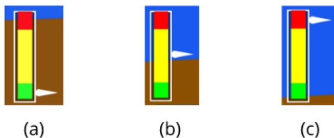
Accordingly, the border between the red and yellow represents the calibrated warning angle.
