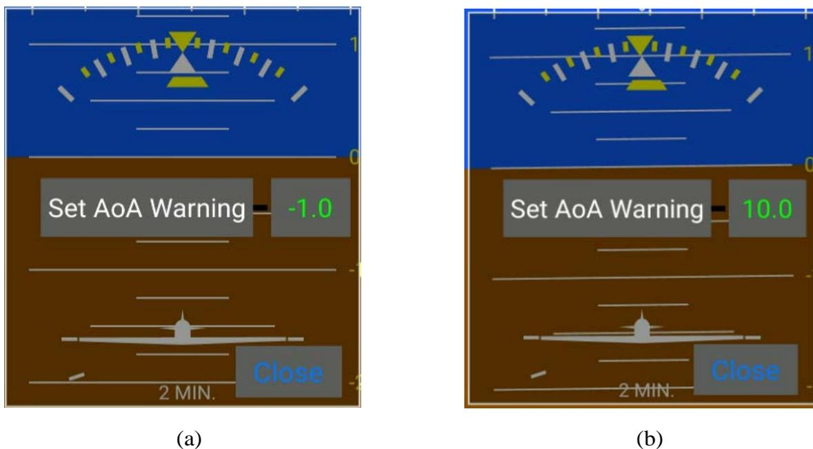
Figure 7: (a) Uncalibrated FlySense device. (b) Calibrated FlySense device (i.e. stall angle has been determined at  $12^\circ$  and accordingly warning angle has been set at  $10^\circ$ ).
