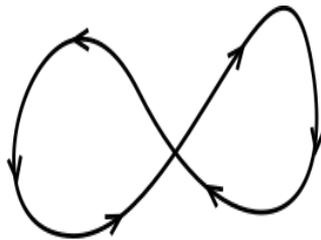
Fig. 5: To easily calibrate the Compass start by slowly rotating FlySense AoA three times around each axis and then perform a sequence of “lazy eight” maneuvers until you have a “Good” or a “Strong” indication on the EFIS TA app.
