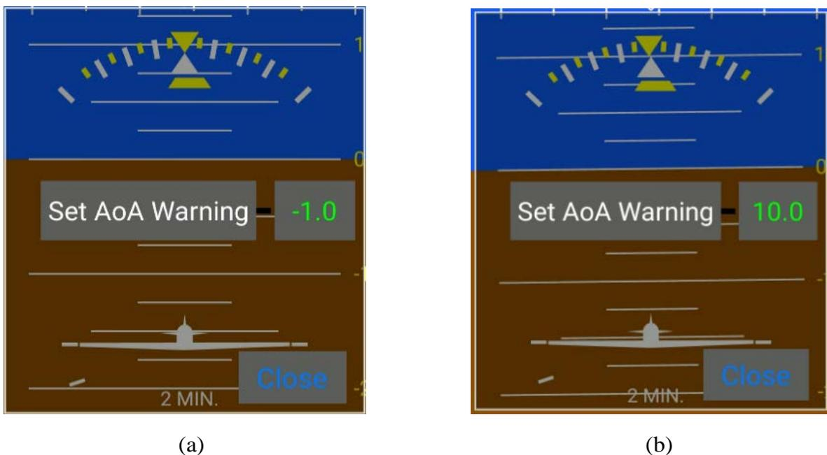
Figure 7: (a) Uncalibrated FlySense device. (b) Calibrated FlySense device (i.e. stall angle has been determined at 12° and accordingly warning angle has been set at 10°).
