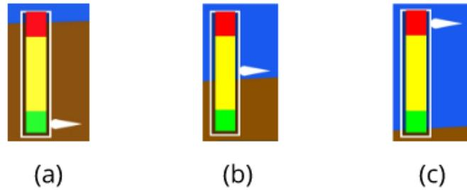
For visual indication purposes, FlySense AoA uses a moving white pointer on the color-bar that indicates the actual AoA. This is illustrated below in Figure 9 that shows three (3) example cases of AoA during flight. The case in Figure 9(c) is a critical case, where the aircraft is close to stall attitude. Figure 9: (a) AoA Normal area. (b) AoA warning area. (c) AoA critical area.
